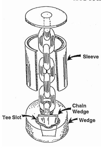
Place the chain in the tee slot of the wedge between the 1st and 3rd link. Then place the chain wedge at the top of the tee slot. Tap slightly to lock in place. Loosely draw the wedge up into the bottom of the sleeve – be certain the wedge is positioned squarely.
