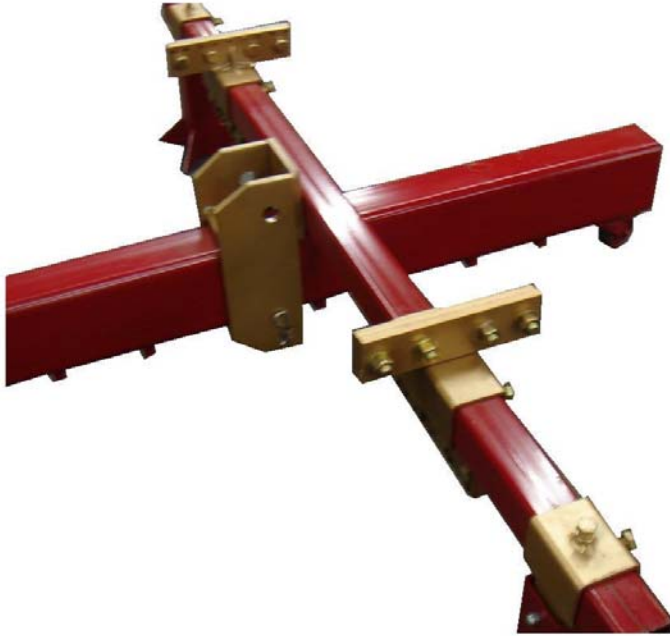
FIGURE 9 - FRONT PULL ON PINCHWELD BODY - NOTE CLAMP ORIENTATION AND LOW POSITION ON PUSHER BRACKET
